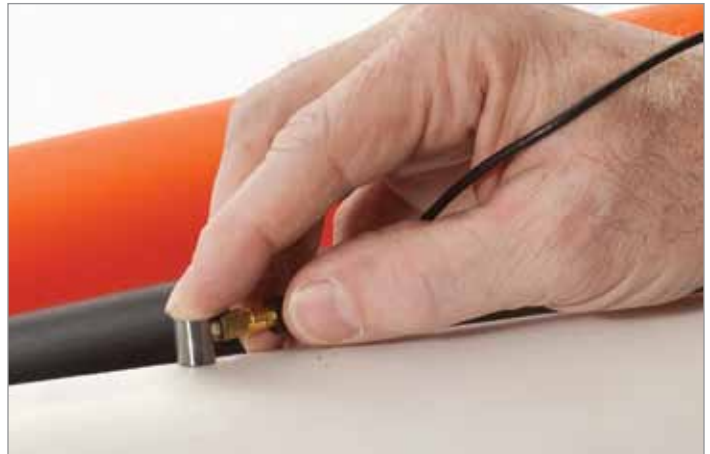
Measure the thickness of many materials including plastic, metal, rubber, glass, ceramic, and composites.
