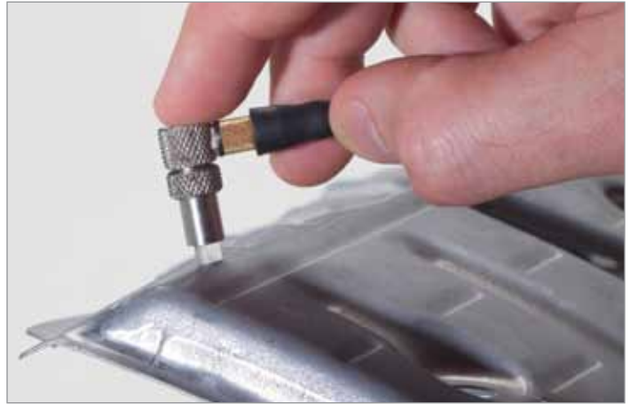
Measure metal thinning caused by bending or forming.
