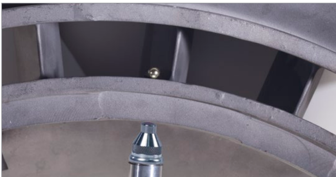
Measurement of a 24.1 mm (0.950 in.) aerospace casting
