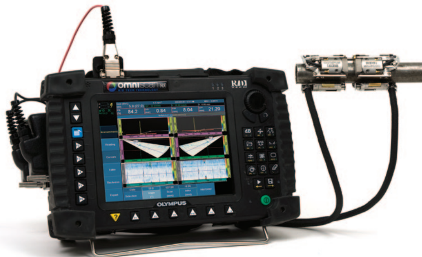
The COBRA scanner on a 0.84 in. pipe with two PA probes and an OmniScan MX 16:128 displaying two PA groups with sectorial scans, A-scans, and C-scans.
