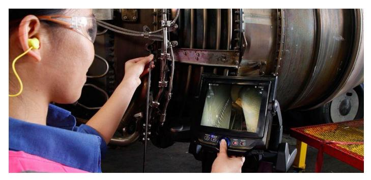
In the power generation, oil gas, and chemical industries, reducing the downtime of rotating machinery such as turbines is a key factor for plant efficiency and profitability. The use of the latest videoscopes with a wide field of view, expanded measurement capabilities, and easy-to-use software enables inspectors to obtain detailed images and measurements quickly and make their inspections more efficient for maximized uptime.
