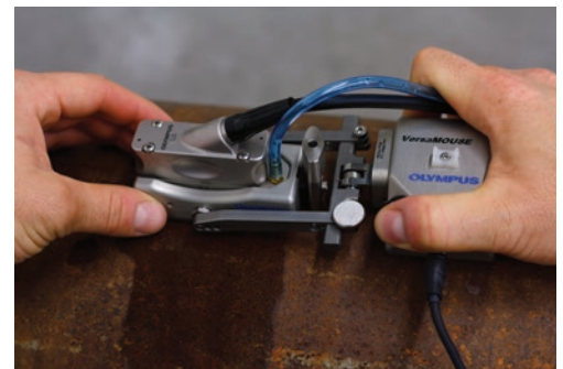
VersaMOUSE scanner and RexoFORM for corrosion inspection.
