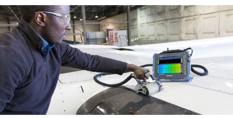
Olympus introduces the RollerFORM™, a new phased array wheel probe designed to address the inspection of composites and other smooth-surfaced materials, such as those commonly used by the aerospace industry. An affordable and easy-to-implement replacement for full 2-D encoding systems, the RollerFORM also offers a viable alternative to immersion techniques.
